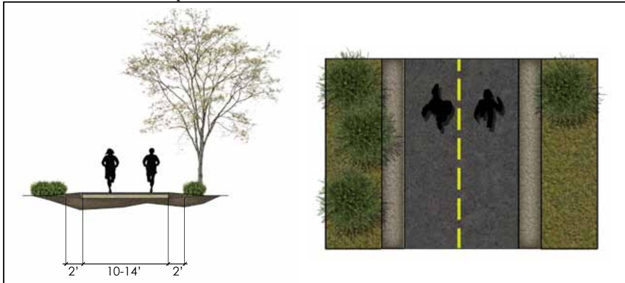
Figure 32: Typical cross section (left) and plan view (right) of an improved multi-use trail.
