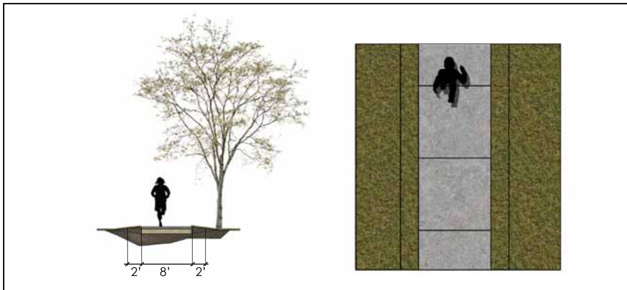
Figure 34: Typical cross section (left) and plan view (right) of an improved pedestrian trail.
